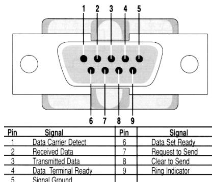
RTS & DTR are outgoing handshaking lines that we can set and hold. DCD, DSR, CTS, and RI are incoming handshaking lines that we can read. RX & TX are controlled by the serial port hardware and pass
