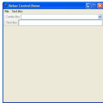
As you can see, a rebar control is just a parent window for different *bands*, which each contain a child control and a text label. They can be moved or resized by the user. By themselves, rebar controls are pretty much useless. But with the help of a child window, they can be much, much more.
